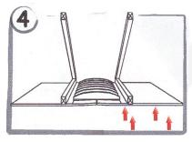
Attach the adjoining plasterboard sheet until it butts up with the other. Fix the sheet to PROfix. See Fig 3.
