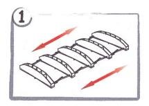
Pull to fully extend PROfix connector and lock in tabs.
