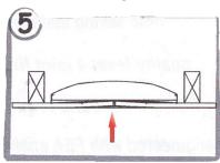
Tape butt joint and fill in flase recess until base and top coat are level with plasterboard.
