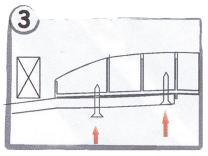
Mount the PROfix connector to the first sheet at approxmately 25mm and 100mm from the butt joint. For added strength, place backblocks between PROfix connector.
