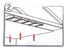
Attach the first plasterboard sheet with the joint midway between joints/trusses.
