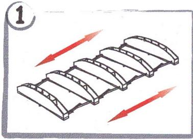
Pull to fully extend PROfix connector and lock in tabs.
