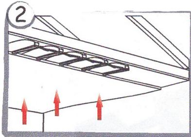
Attach the first plasterboard sheet with the joint midway between joints/trusses.
