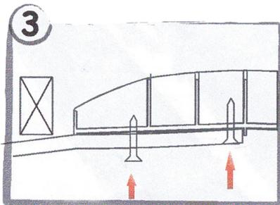
Mount the PROfix connector to the first sheet at approximately 25mm and 100mm from the butt joint. For added strength, place backblocks between PROfix connector.
